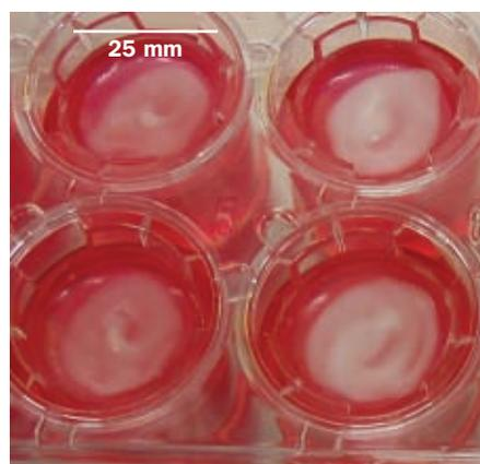
**Figure 2:** Direct application of skincare products onto LabSkin. The size (4.5 cm<sup>2</sup>) and strength of the material allows 'real-world' application protocols to be used i.e. twice daily, for 5 days using a fingertip.
